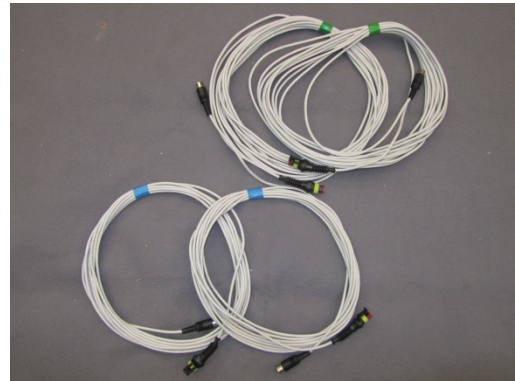
Connection cables for mechanical limit switch
